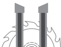
**Alternate top bevel saw blade (W/PW)**
