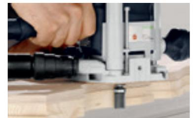
**Turning plate edge trimming cutter HW with ball bearing guide, shank 8 mm**
