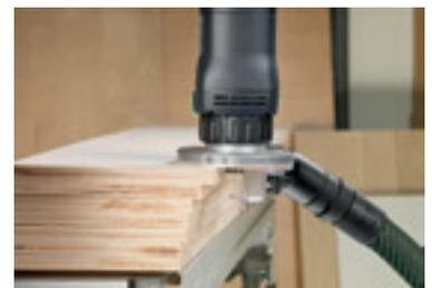
Chamfering plastic or solid wood veneer.
