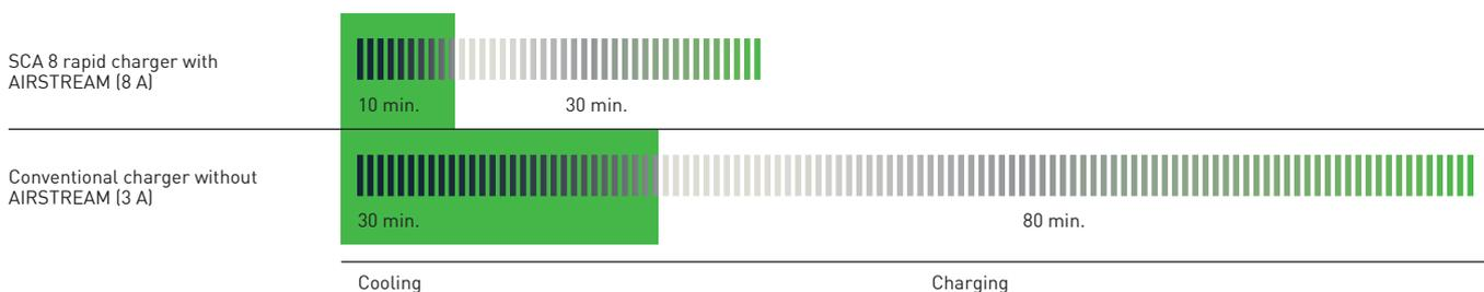
Specifications apply to the 5.2 Ah AIRSTREAM battery
